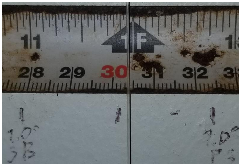
Figure 6-6: Pedulum Reading 30.4 cm (0.16 deg to PS) - Vessel Post-Operational condition
