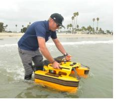
This device allows Marine Bureau staff to efficiently remove small water debris that would otherwise require a boat and additional staffing to drive and net the debris manually. With the Jellyfishbot, one staff member can both remotely operate the device and remove debris. Additionally, the size of the device allows
